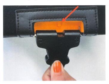
The charging socket is on the right-hand side of the battery beneath the Velcro flap. When you plug the charger into the mains, it will show a green light. When plugged into the battery it will turn red. Once charging has been completed, the light will show green.
