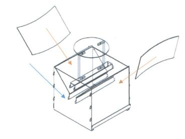
4 Attach the light board then affix the rain guard top. Note: the light board is formed to its correct shape when slotted into position. Once your trap is formed screw in the bulb (do not screw in by holding the glass envelope but by its base) TO MOVE THE TRAP, LIFT BY THE SIDES WHERE THE LIGHT BOARD ATTACH, THIS WILL KEEP THE TRAP ALL TOGETHER NEATLY
