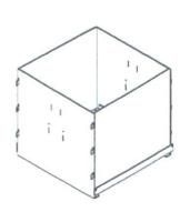
2 Insert the two thin pieces of polycarbonate by bowing slightly then sliding into place.
